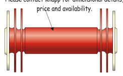
To ensure passage through a sub-sea wye fitting, it is necessary for a disc-type pig to be longer than normal. Its' front discs must make a seal in the run of the wye while the rear discs maintain a seal in the lateral of the wye
